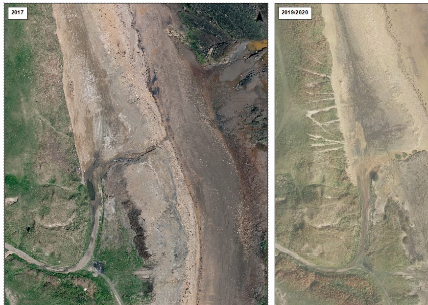
Figure 2-7 – Erosion of colliery spoil beach in Lynemouth Bay, 2017 (left) and 2019-20 (right)
