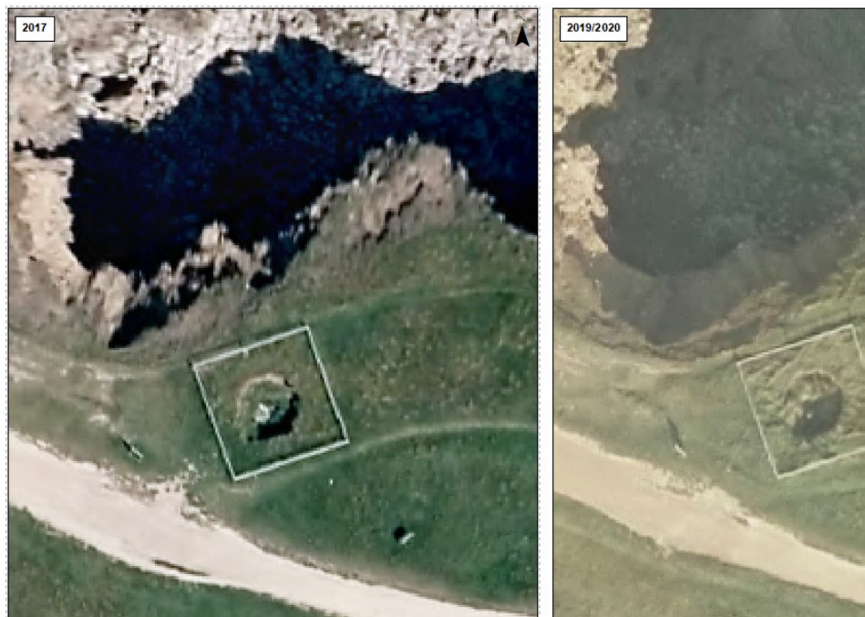
Figure 2-16 – Sink hole at Man Haven, 2017 (left) and 2019-20 (right)
