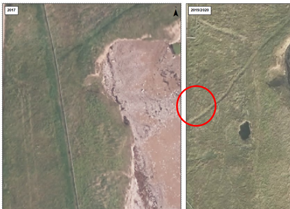
Figure 2-18 – New sink hole at Whitburn Coastal Park, 2017 (left) and 2019-20 (right)
