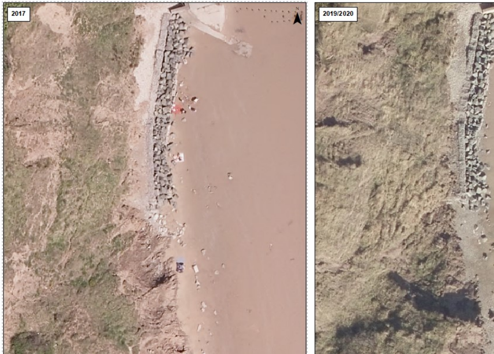
Figure 2-25 – Outflanking at end of Filey Seawall
